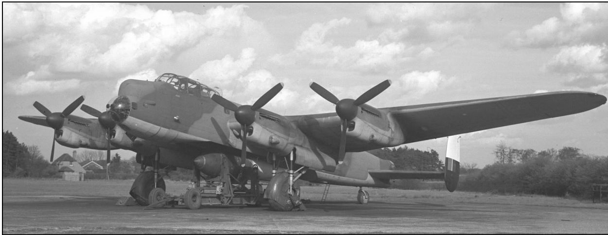
A modified Lancaster is seen above with a TALLBOY bomb being mounted in the bomb bay. The nose turret has been deleted to save weight and improved Rolls-Royce Merlin engines have been fitted, along with other modifications. - RCAF Photo PL-446097
