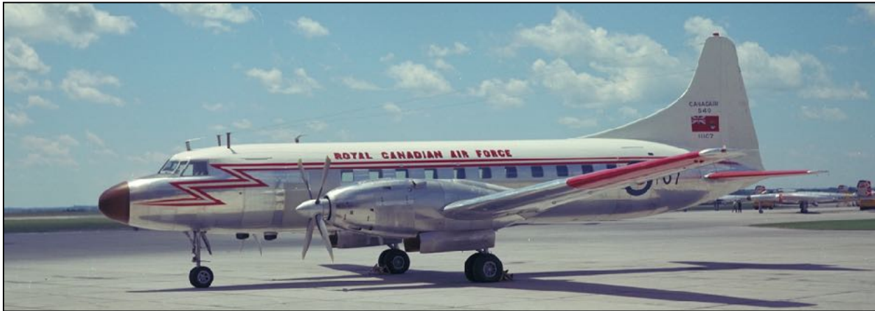
Above - This is an example of the Canadair-built CC-106 Cosmopolitan in its original Napier-Eland engine configuration that proved highly unsatisfactory in terms of performance and reliability. - (RCAF Photo PCN-995)
