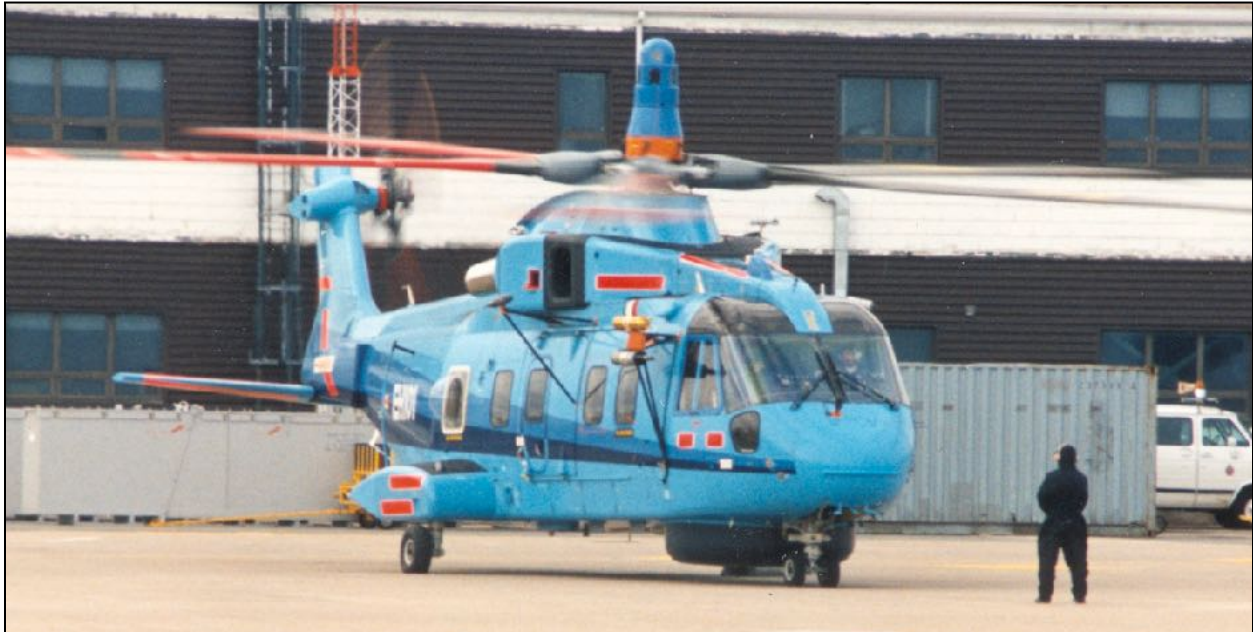
Above - This is an EH-101 test aircraft in Halifax, NS for icing tests. It was intended to become the the CH-148 Petrel. - (Author's Photo)
