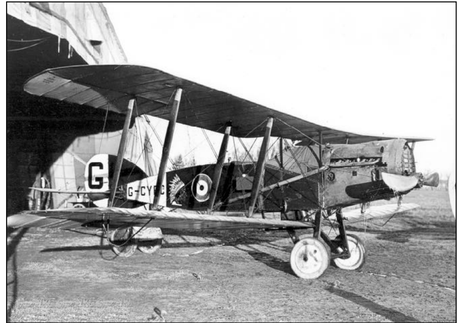
Note the variation in the Air Board markings of this Bristol F2B Fighter, G-CYBC , with comparatively small fuselage letters placed well aft and the wartime markings and roundels still being displayed. - (CF Photo)
