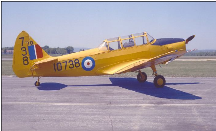
This example of a Fairchild Cornell trainer illustrates the classic BCATP colours: yellow overall with prominent registration numbers, A-type roundels in all positions and an anti-glare black section forward of the cockpit – (CF Photo)
