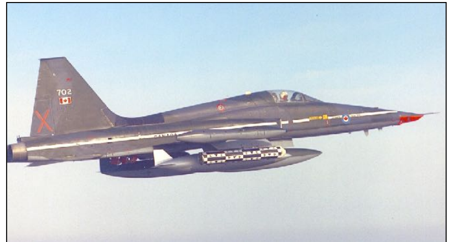
AETE CF116702 wears various black and white markings which serve as photographic reference points; in this case the markings have also been extended to the underwing stores under test – (CF Photo)
