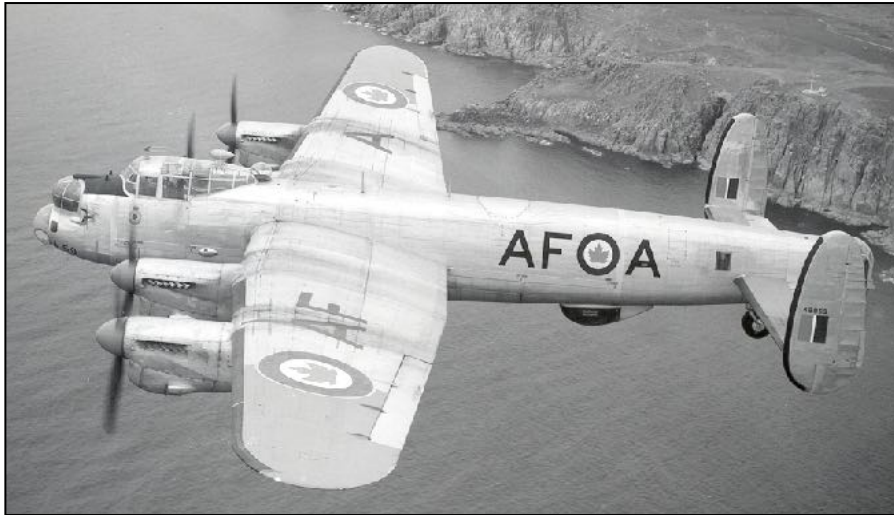
An example of the VC era markings: This post-war Lancaster has been converted to the Mk 10 MR (Maritime Reconnaissance) variant. The aircraft is coded AF*A and its registration under ICAO system was therefore VC-AFA. - (CF Photo)
